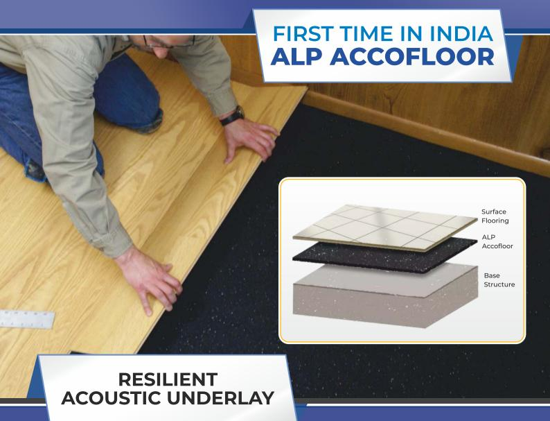
ALP ACCOFLOOR Acoustic Underlay has been specifically designed to help reduce airborne and impact noise within a floor system. It is essentially a resilient rubber layer that is installed underneath the final floor finish isolating / decoupling the flooring from the structure of the building.
